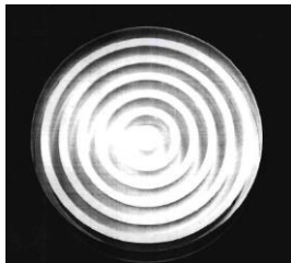
Eljen EJ-410P ZnS(Ag)-filled rings surrounded by lucite
