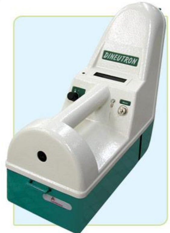
Canberra DiNeutron : Uses two PE-moderated detectors
