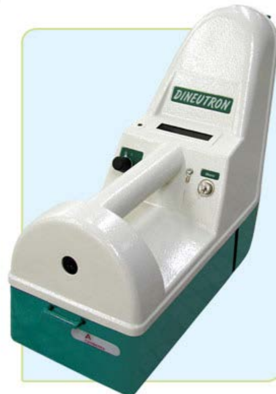
Canberra DiNeutron : Uses two PE-moderated detectors
