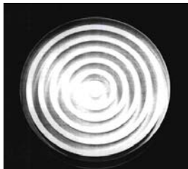
Eljen EJ-410P ZnS(Ag)-filled rings surrounded by lucite
