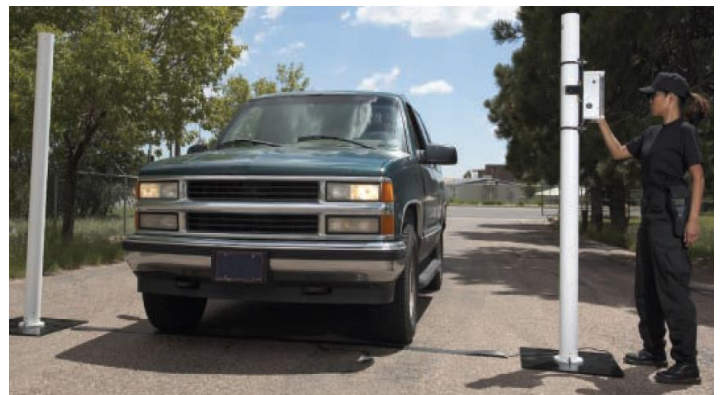
Figure 3. A vehicle chokepoint using a PRPM Photo courtesy of Thermo Scientific, Inc.
