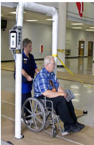
Figure 2. A PRPM in use at a community reception center Photo from Resource 1
